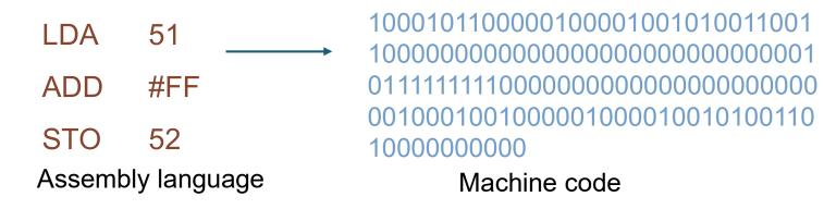
means "Load the contents of memory location 51 into the accumulator, add hexadecimal value FF and store the result in location 52"
